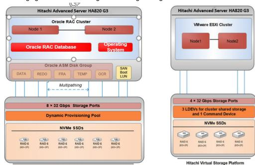
The following figure illustrates the high-level storage configuration for this solution.
