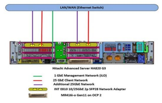
The following figure shows the topology of this reference solution using external drives on a storage system, such as Hitachi Virtual Storage Platform E1090.
