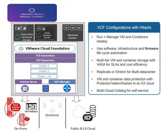
VMware Cloud Foundation (VCF) supports Hitachi SAN storage (vVols prior to VCF 9, and VMFS) used as principal or supplemental storage. The use cases vary by implementation, ranging from flexibility to scale storage footprint, mission critical applications with stringent RPO/RTO requirements, to simply matching business outcomes to suitable tier of storage.
