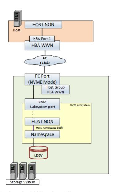
Conventional Fibre Channel and iSCSI requires an LU mapping for a port to manage an access route between the host and the logical volume. NVMe-oF, on the other hand, requires the following system components to be configured on the storage system between the host and the logical volume.
