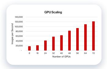
The final set of performance tests measures Hitachi Content Software for File's ability to deliver performance to a single GPU server utilizing GPUDirect Storage. Hitachi Content Software for File scaled performance inside a single NVIDIA DGX-2™ GPU server from one 100Gbit EDR link to 8 EDR links with linear scaling, saturating the network bandwidth.
