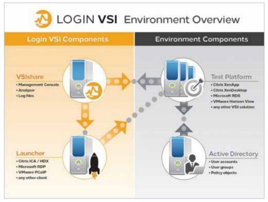
When used for benchmarking, the product measures the total response times of several specific user operations being performed within a desktop workload, in a scripted loop. The baseline is the measurement of the specific operational response times performed in the desktop workload, measured in milliseconds (ms). Two values are very important: VSIbase and VSImax.
