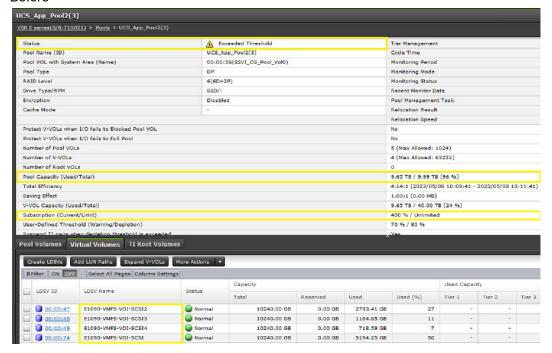
Prior to enabling the capacity saving function for both deduplication and compression on the Hitachi Virtual Storage Platform, the VSP pool exceeded capacity thresholds and had a Used/Total capacity of 9.65 Tb of 9.99 Tb.
