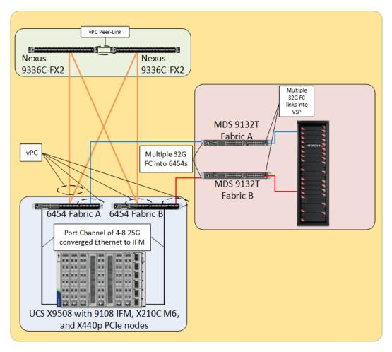
The Cisco UCS X210c M6 nodes in this topology are hosted within a Cisco UCS X9508 chassis and connect into the fabric interconnects from the chassis using the Cisco UCS 9108 IFM. The 9108 IFM supports 25 G connections into the 10/25 G ports of the Cisco UCS 6454 FI, delivering a high port availability that may fit well in a branch office setting.
