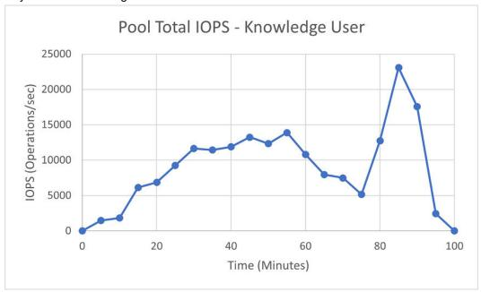
Hitachi Virtual Storage Platform showed sub-millisecond response times during knowledge user testing. During peak log on period the VSP provided a max total response time of .38 milliseconds, while during steady state and log off period performance improved to .24 milliseconds.
