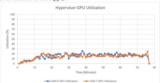
During power profile testing with GPUs, both hypervisors showed an average utilization of 18% as indicated in the following graph.
