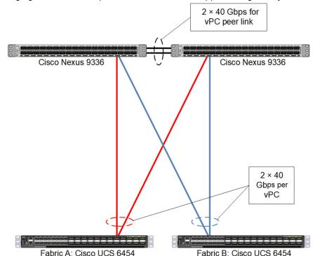
The following figure shows the upstream network for the application gateway:
