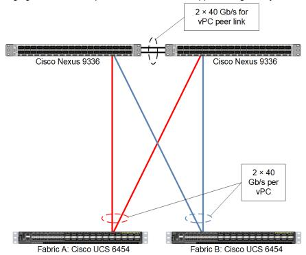
For the SAP HANA nodes, you need to make network connections to the Cisco Nexus 9336 switches or to other external switches. Bond the corresponding two ports, ethX and ethY, as bond0 at the operating system level using the active-active network bond mode with the following options:
