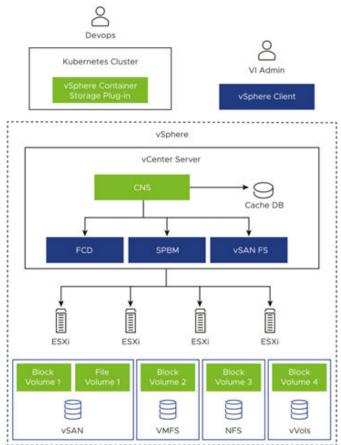
Deployment of Openshift worker nodes on VMware vSphere requires installation of the vSphere CSI driver to take advantage of the vSphere SPBM to Kubernetes StorageClass mapping.
