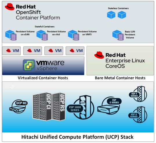
You can deploy OpenShift on bare metal hosts and/or virtual hosts or both. In some cases, the master nodes are virtualized while the worker nodes can be hybrid bare metal and virtual nodes. Depending on the deployment purposes, different deployments can be used. For this reference architecture, the OpenShift clusters use a hybrid deployment, combining bare metal and virtual worker nodes to show the benefits of both types of deployments.
