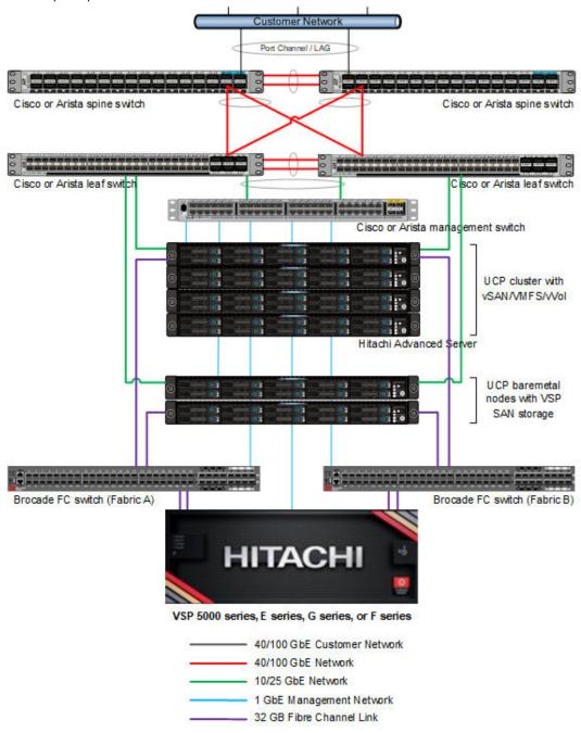
The configuration with Hitachi Virtual Storage Platform is described in Unified Compute Platform CI/HC/RS in <u>HitachiUnified Compute Platform CI for VMware vSphere Reference</u> <u>Architecture Guide</u>.
