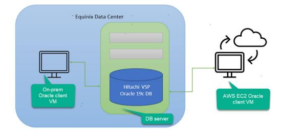
The following figure shows a high-level reference diagram for this cloud solution.
