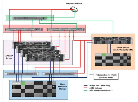
The following figure shows an overview of the landscape including the VMware server and its storage, and all network and Fibre Channel connections.
