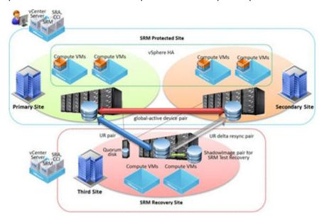
Installing VMware Site Recovery Manager in this 3DC environment gives you the orchestrated and repeatable planned or unplanned migration or disaster recovery operations using a tested and proven recovery plan. This enables end-to-end virtual machine protection across 3 data centers. As a normal state, VMware VLSR protects the virtual machine between the primary and the third data center.
