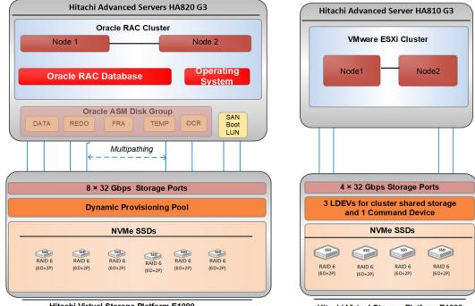
The high-level storage configuration diagram for this solution is shown in following figure.
