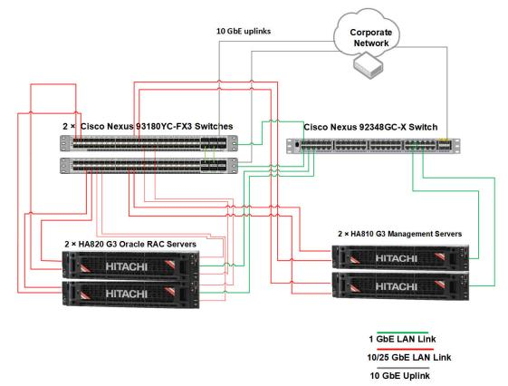
The following figure shows the IP network switch connection.
