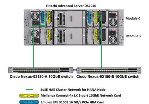
Configure the SUSE Linux Enterprise High Availability Extension or Red Hat Enterprise Linux High Availability cluster network using operating system level bonding on every node.
