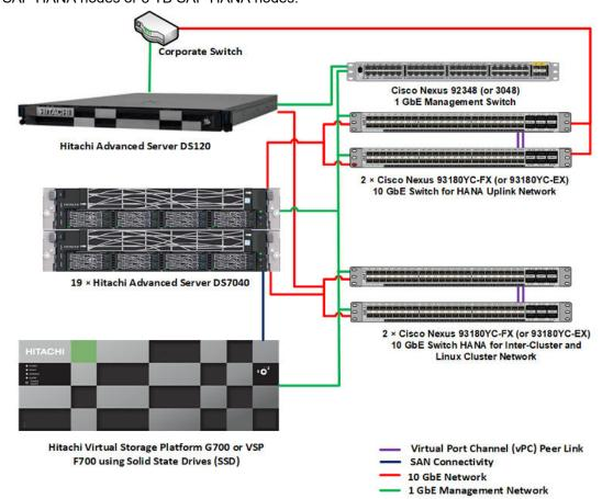
The following figure shows the solution overview for the scale-out configuration using 1.5 TB SAP HANA nodes or 3 TB SAP HANA nodes.
