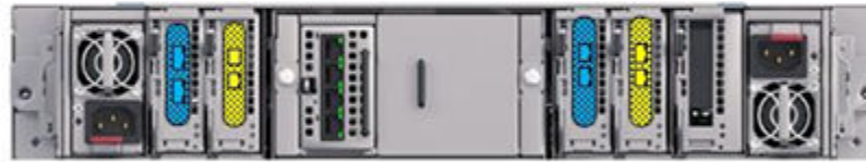
Hitachi Advanced Server DS7000 with external Storage (Back)
