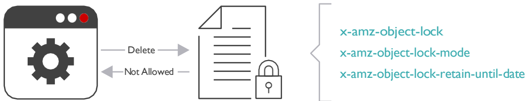
Figure 4. Immutable backup: The Hitachi and Veeam solution prevents a backup object from being deleted.
