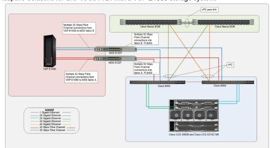
The following figure shows the topology of this architecture for Cisco UCSX and Hitachi Adaptive Solutions for SAP HANA TDI with a VSP E1090 storage system.
