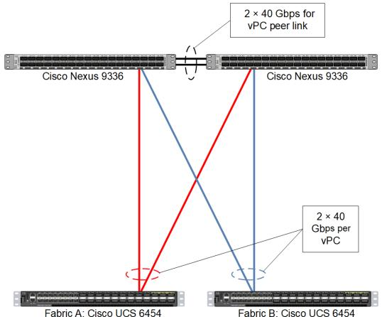
For the SAP HANA nodes, you must make network connections to the Cisco Nexus 9336 switches or to any other external switches. Bond the corresponding two ports, ethX and ethY, as bond0 at the operating system level using the active-active network bond mode with the following options:
