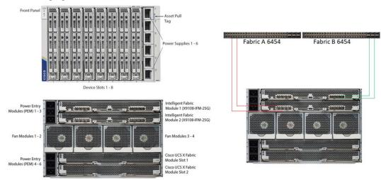
The <u>Cisco UCS 9108 25G Intelligent Fabric Modules</u> connects the I/O fabric between the Cisco UCS 6454 Fabric Interconnect and the Cisco UCS X9508 Chassis, enabling a lossless and deterministic converged fabric to connect all blades and chassis together.
