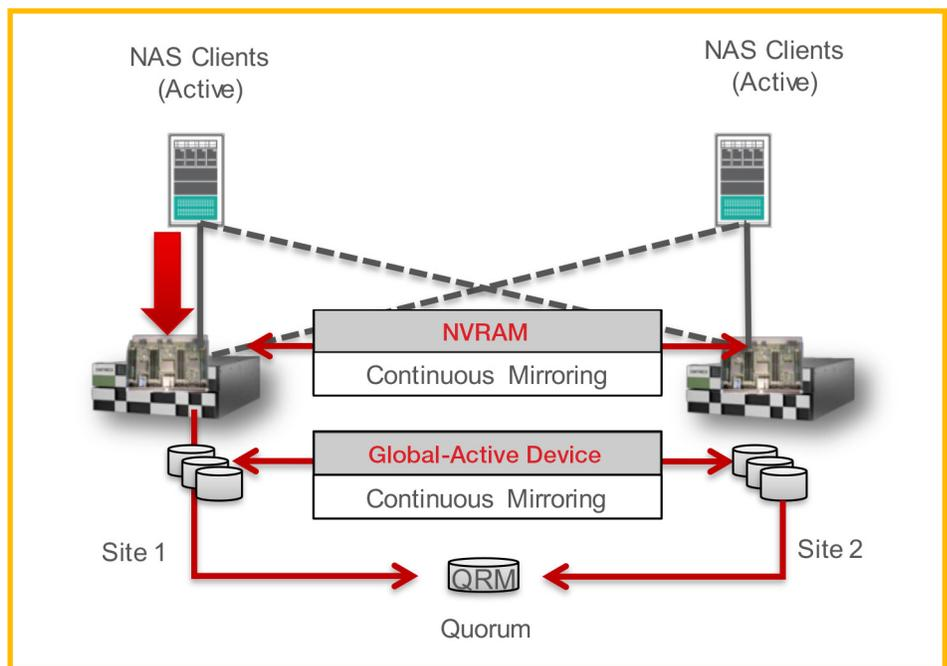
Figure 2. Global-Active Device Enhanced for NAS High-Level Architecture
